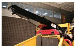
FEED YOUR WAY. The patented winch boom design can be raised out of the way when mechanically feeding the machine for optimal visibility and feeding access.
