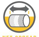
Little net stretch with optimum net spread to cover square-shouldered bales from one side to the other.
