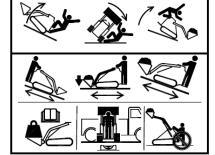
**WARNING:** Traveling on slopes or with load elevated may result in tip over. Serious crushing injury or death can result.
