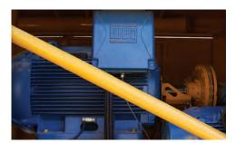
**ELECTRIC MOTORS.** Equipped with a 500 hp (373 kW) WEG totally enclosed fan-cooled electric motor to power the mill. A separate 60 hp (44.7 kW) electric motor powers the pump for the hydraulic circuits, while a 2 hp (1.5 kW) electric motor powers the fan to cool the hydraulic system.
