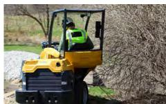
COMPACT SIZE. With a narrow tire option, the ATX530 is 38.6-in (98-cm) wide, while the standard tires make the machine 47.2-in (120 cm) wide. The standard length of the ATX530 is 102.1 in (260 cm).
