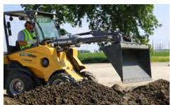
TELESCOPIC BOOM. The telescopic boom on the ATX530 extends 29.1 in (73.9 cm) for loading materials to a dump height of 108.3 in (275.1 cm) in hinge pin height. The telescopic boom can also aid in dumping material over the backside of a retaining wall or grabbing material over an obstruction.
