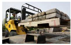
LIFT-CAPACITY-TO-WEIGHT RATIO. The ATX530 has a rated operating capacity (straight) of 1,343 lb (609.2 kg)\* while having a standard weight of 2,760 lb (1,252 kg) with rear weights and without attachments. This lift-capacity-to-weight ratio allows contractors to utilize a lighter machine while still being able to carry heavy materials on the jobsite.
