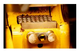
PATENTED, SLIDING, OPEN-SIDE VISE. Minimize the number of steps to change out a rod with this patented vise design. The vise utilizes sliding, openside functionality, which allows you to see the rod joint.
