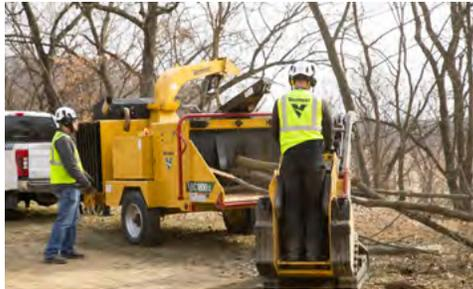
**CHIPPING PRODUCTIVITY.** The patented Smart-Feed system monitors engine rpm and automatically stops, reverses and re-engages the feed rollers when feeding larger material.
