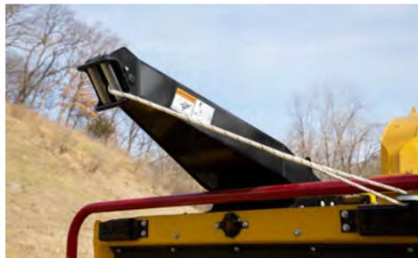
**OPTIONAL WINCH.** The winch allows operators to move large logs with less effort. The 150-ft (91.4 m) winch line has 2,000 lb (907.2 kg) of pulling force.
