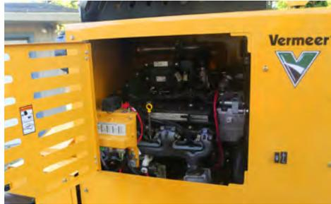
**165-HP INDUSTRIAL GAS ENGINE.** The BC1800XL is designed with a 165-hp (121-kw) PSI 5.7 L gas engine, powerful enough to tackle jobsite challenges when chipping large diameter wood.
