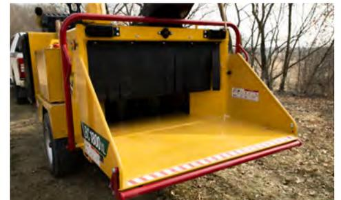
**OPERATOR SAFETY.** Mounted over the feed table, the four-position upper feed control bar enables the operator to stop the feed rollers and select forward or reverse. The patented bottom feed stop bar is strategically located to make it possible for an operator's leg to strike the bar and shut off the feed mechanism.
