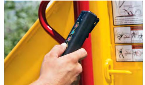
**TAKE CONTROL.** With the optional Tree Commander™ remote control, jobsite productivity can be improved by allowing the operator to control brush chipper functions remotely. The remote can be attached to the operator's belt or held in an optional bracket mounted directly to the operator's station of a Vermeer compact utility loader.
