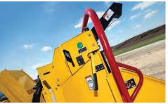
**EASILY LIFTS HEAVY MATERIAL.** An optional winch allows operators to move large logs effortlessly. The 150' (45.7 m) winch line can handle logs up to 2000 lb (907.2 kg) and can be used to lift the log onto the feed table.
