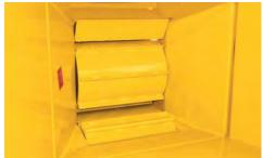
**DUAL HORIZONTAL OFFSET FEED ROLLERS.** Improve performance by aggressively grabbing and feeding material to the drum. The offset helps the upper feed roller climb over big logs or material with lots of branches and forks.
