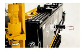
DRILL LONGER IN HARDER GROUND CONDITIONS. Optional class-leading rod capacity to bore further with 480 ft (150 m) of rod on board without having to get off the machine. A 45-gpm (170-L/min) mud pump increases fluid flow rate, helping you ream quickly and pull large product faster.
