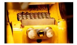
**PATENTED, SLIDING, OPEN-SIDE VISE.** Minimize the number of steps to change out a rod with this patented vise design. The vise utilizes sliding, open-side functionality, which allows you to see the rod joint.
