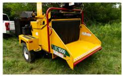
**OPERATOR SAFETY.** Mounted over the feed table, the four-position upper feed control bar enables the operator to stop the feed rollers and select forward/reverse. The patented bottom feed stop bar is strategically located to make it possible for an operator's leg to strike the bar and shut off the feed mechanism.
