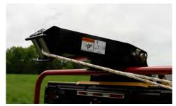
**EASILY LIFT HEAVY MATERIAL.** An optional winch allows operators to move large logs effortlessly. The 150-ft (45.7-m) winch line can handle logs up to 2,000 lb (907.2 kg) and can automatically lift the logs onto the feed table.
