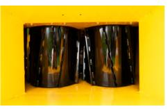
SMOOTH FEEDING. Vertical feed rollers with helical cleats help hold material firmly to the infeed table, which helps reduce vibration, shock and structural loading to the rear of the machine.
