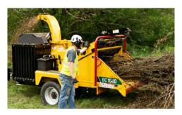
ENGINE OPTIONS. The BC1500 is offered in either a 172-hp (128-kW) Origin 6.2 L gasoline engine or a 130-hp (97-kW) Cummins QSF 3.8 L Tier 4 Final engine.
