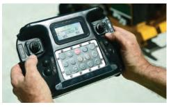
**REMOTE CONTROL.** A remote control gives you 360-degree control of the machine, providing greater maneuverability on tight jobsites, as well as visibility to the complete worksite and to avoid potential obstacles or obstructions that may be difficult to operate with conventional controls.
