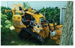
**COMPACT SIZE.** A narrow width of 34.5 in (87.6 cm) and length of 81 in (205.7 cm) allows you to enter gated yards and install utilities in tight jobsites.
