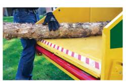
**ELECTRONICALLY SWITCHED BOTTOM FEED STOP BAR** is strategically located to make it possible for the operator's leg to strike the bar and shut off the feed mechanism either intentionally or automatically in an emergency situation increasing operator safety while feeding material.
