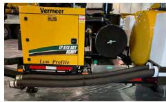
SIDE HOSE AND TOOLING (SHT) STORAGE (OPTION). The new SHT package allows for 60 ft (18 m) of suction hose storage on a trailermounted unit. This doubles the traditional 30-ft (9-m) hose storage on all other brands.
