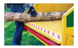
**ELECTRONICALLY SWITCHED BOTTOM** FEED STOP BAR is strategically located to make it possible for the operator's leg to strike the bar and shut off the feed mechanism either intentionally or automatically in an emergency situation increasing operator safety while feeding material.
