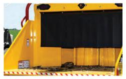
A LARGE RECTANGULAR 12 IN X 17 IN (30.5 CM X 43.2 CM) FEED OPENING. Helps with productivity by reducing the need to trim material before feeding it into the chipper.
