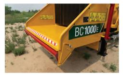
**BUILT WITH OPERATOR SAFETY IN MIND.** Through the patented bottom-stop feed bar which is located along the bottom of the feed table. This system makes it possible for an operator to strike the bar and shut off the feed mechanism. Dual reset/hold-to-run buttons allow the operator readily reset the bottom-stop feed bar.
