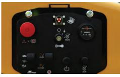
**THE CONTROL PANEL.** Fully weatherproof and contains a Siemens soft starter which helps protect the drum motor from overloading and voltage dips from the power grid.
