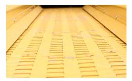
STEEL INFEED CONVEYOR CHAIN WITH DUAL-DRIVEN ROLLER.
