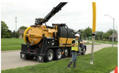
PTO DRIVE SYSTEM. A side PTO drive system allows the vac to keep running while moving the truck between holes, rather than requiring full machine shutdown for each move.
