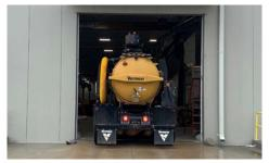
LOW PROFILE. Low overall height of 11.5 ft (3.51 m). Drive under a 12-ft (3.66-m) shop door or bridge with comfort. Plus, one of the lightest 8-yd3 (6.1-m3) trucks in the industry to maximize payload.
