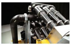
**CLEANING EFFICIENCY.** Premium cleaning performance is achieved through six 4-in (10-cm) long-body hydrocyclones in combination with a relatively large screen area.
