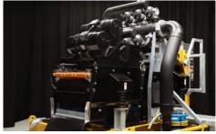
**CONTINUOUS PERFORMANCE.** The robust design of the shaker deck delivers stable performance under variable processing volume. A high capacity 15-hp (11-kW) pump is used for optimal circulation.
