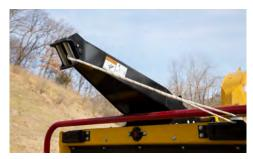
**OPTIONAL WINCH.** The winch allows operators to move large logs with less effort. The 150-ft (91.4 m) winch line has 2,000 lb (907.2 kg) of pulling force.
