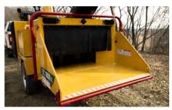
**OPERATOR SAFETY.** Mounted over the feed table. the four-position upper feed control bar enables the operator to stop the feed rollers and select forward or reverse. The patented bottom feed stop bar is strategically located to make it possible for an operator's leg to strike the bar and shut off the feed mechanism.
