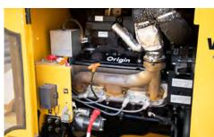
172-HP INDUSTRIAL GAS ENGINE. The BC1800xL is designed with a 172-hp (128-kw) Origin 6.2 L gas engine, powerful enough to tackle jobsite challenges when chipping large diameter wood.
