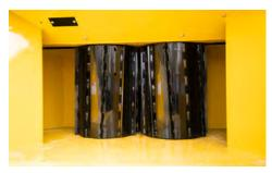
SMOOTH FEEDING. Vertical feed rollers with helical cleats help hold material firmly to the feed table, which helps reduce vibration, shock and structural loading to the rear of the machine.
