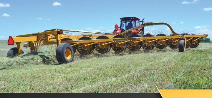
The VR1428 and VR2040 high-capacity wheel rakes from Vermeer are built tough to handle heavy crops efficiently — with ease of maintenance in mind. A unique center splitter attachment lets you cover the entire swath — up to 40 ft (12.2 m) wide. Plus, hydraulic suspension on each wheel and a select frame design provide serious flexibility in the field. Flex some serious muscle this haying season.
