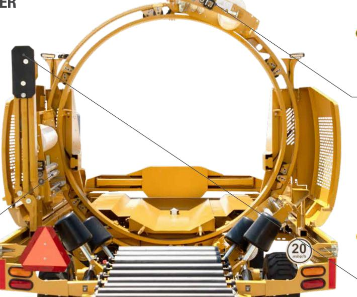
Have peace of mind knowing an optional film break sensor is constantly watching film so you don't have to. It senses the film once it's applying, makes sure bales are covered with the intended number of wraps and automatically shuts down the machine if the film breaks.
