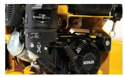
QUICK YIELD TIME. Equipped with a Rehlko 7-hp (5-kW) engine for high productivity to get drilling quickly.
