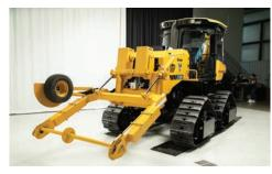
5,000-LB REEL CARRIER ATTACHMENT **OPTION.** On the tractor equipped with a plow, add a reel carrier attachment capable of carrying up to 5,000 lb (2,268 kg) of product.
