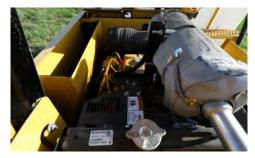
POWERFUL PERFORMANCE. The MX300D is equipped with a 24.7 hp (18.4 kW) CAT C1.1 engine and 350-gpm (1,324.9-L/min) pump flow to provide powerful performance on the job.
