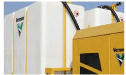
**CONVENIENT CONFIGURATION.** There are two tank options for the MX300D that are powered by the same power unit, to provide more fluid onsite, with the option to support either the 750-gal (2,839.1-L) or the 1,000-gal (3,785.4-L) tank. The tanks can run independently, or together, depending on fluid amount needed.
