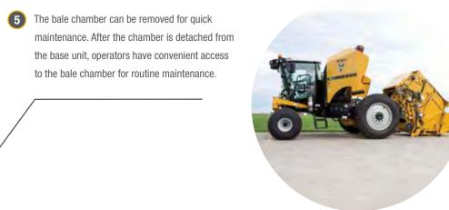
6 By automating parts of the baling process, the ZR5-1200 helps reduce the number of manual steps to make a bale to just one step. When you choose to bale in automatic mode, the ZR5-1200 control system, paired with a hydraulic drive system, can make real-time adjustments based on field and crop conditions and can even open and close the tailgate automatically.
