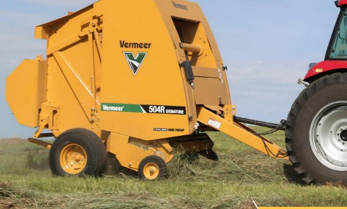
The Signature name says it all. The 504R Signature baler advances the Vermeer legacy by giving the working man a baler and is built upon the three signature pillars of Vermeer balers — convenience, ease of use and durability. Combine that with a camless wide pickup, rotor and durable steel windguard roller for quiet and smooth operation — all while making bales at a quick pace. Backed by a 3-year pickup warranty\*, it's clear the 504R Signature baler is truly one of a kind.
