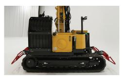
**WORK IN TOUGH GROUND CONDITIONS AND** ON A VARIETY OF JOBSITES. Up your machine utilization and open more bid opportunities with a 25-ft (7.6-m) pile driving capability and 10-in (30cm) pile reveal capability. Offered with a hammer as standard or optional rotary attachment.
