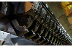
**DOUBLE-ENDED COMB TEETH.** The LS3600 has individual bolt-in comb teeth that have two usable edges. This helps extend the life of your teeth and minimize wear costs.
