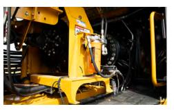
**MECHANICAL DRIVELINE AND PROTECTION.** Equipped with a reversable mechanical transmission for an efficient power transfer that maximizes productivity. A torque limiter automatically disengages the drive when max torque is experienced – helping protect critical machine components.
