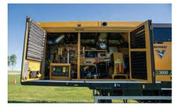
**ENGINE BAY ACCESS.** The LS3600 gives you unparalleled access into the machine. The maintenance-friendly and highly accessible engine bay design includes large access doors, multiple ladder points and a large service platform to help with ease of maintenance and serviceability.
