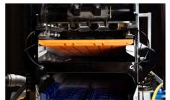
QUICK-CHANGE SCREENS. The primary screens are kept in place with an air-clamping system, powered by an onboard air compressor. This allows for ease of access and the ability to quickly change the screens.
