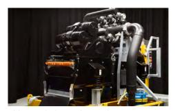
**CONTINUOUS PERFORMANCE.** The robust design of the shaker deck delivers stable performance under variable processing volume. A high capacity 15-hp (11-kW) pump is used for optimal circulation.
