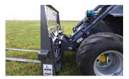
FULL-SIZED ATTACHMENT PLATE. The full-sized attachment plate on the ATX960 is compatible will full-sized articulated loader attachments. The ATX960 can be fitted with various authorized attachments to meet the jobsite need, may that be for snow removal, landscaping, logging and tree care work, or various other applications.
