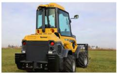
**COMPACT SIZE.** With a narrow tire option, the ATX960 is 52-in (132-cm) wide, while the standard tires make the machine 59-in (149.9-cm) wide. The standard length of the ATX960 is 141 in (358.1 cm).
