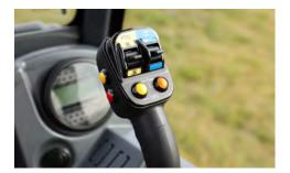
**MULTIFUNCTION JOYSTICK.** The multifunction joystick utilizes electric-over-hydraulic toggles for ease of access to machine functions like the telescopic boom, auxiliary hydraulic controls and the DBS. The operator does not have to remove their hand from the loader arm controls in order to function any of these features.
