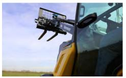
**TELESCOPIC BOOM.** The telescopic boom on the ATX960 extends 31.5 in (80 cm) for loading materials to a dump height of 126 in (320 cm) in hinge pin height. The telescopic boom can also aid in dumping material over the backside of a retaining wall or grabbing material over an obstruction.
