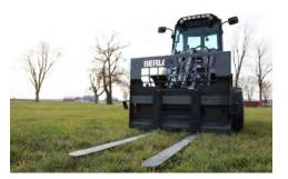
**LIFT-CAPACITY-TO-WEIGHT RATIO.** The ATX960 has a rated operating capacity (straight) of 3,285 lb (1,490 kg) while having a standard weight of 6,040 lb (2,740 kg) with rear and side weights and without attachments. This lift-capacity-to-weight ratio allows contractors to use a lighter machine while still being able to carry heavy materials on the jobsite.
