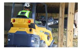
**COMPACT SIZE.** With a narrow tire option, the ATX720 is 42.1-in (106.9-cm) wide, while the standard tires make the machine 50.4-in (128-cm) wide. The standard length of the ATX720 is 114.8 in (292 cm).
