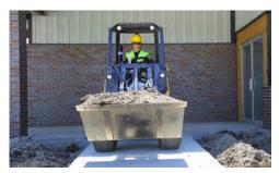
**LIFT-CAPACITY-TO-WEIGHT RATIO.** The ATX720 has a rated operating capacity (straight) of 1,917 lb (870 kg) while having a standard weight of 3,911 lb (1,774 kg) with rear weights and without attachments. This allows contractors to use a lighter machine while still being able to carry heavy materials on the jobsite.
