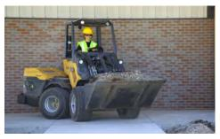
**FRONT-SEATED ARTICULATION.** Front-seated articulation helps the machine work in compact jobsites while keeping turf disturbance a priority.
