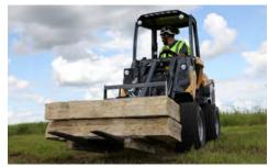
LIFT-TO-WEIGHT RATIO. The ATX850 has a rated operating capacity (straight) of 2,517 lb (1,142 kg) while having a standard weight of 4,587 lb (2,081 kg) with rear weights and without attachments. This lift-capacity-to-weight ratio allows contractors to use a lighter machine while still being able to carry heavy materials on the jobsite.
