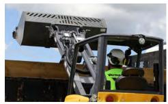
**TELESCOPIC BOOM.** The telescopic boom on the ATX850 extends to 29.1 in (73.9 cm) for loading materials to a dump height of 117.3 in (297.9 cm) in hinge pin height. The telescopic boom can also aid in dumping material over the back side of a retaining wall or grabbing material over an obstruction.
