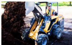
**COMPACT SIZE.** With a narrow tire option, the ATX850 is 42.1-in (106.9-cm) wide, while the standard tires make the machine 50.4-in (128-cm) wide. The standard length of the ATX850 is 124.5 in (316 cm).
