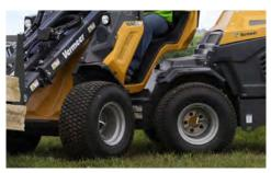
FOUR WHEEL DRIVE HYDROSTATIC DIRECT **DRIVE MOTORS.** As each wheel has a hydrostatic direct drive motor, hydraulic oil can flow freely to each wheel as needed during transport to help reduce ground disturbance on turf when making turns. The four wheel drive hydrostatic direct drive motors also allow for the use of the DBS and torque divider to increase tractive effort in difficult conditions.
